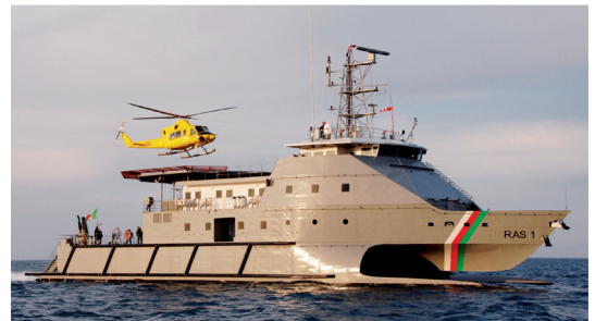
high-speed wave-piercing aluminium catamaran: WPCAT 52 R
