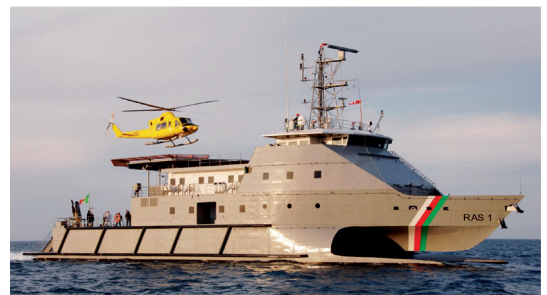
high-speed wave-piercing aluminium catamaran: WPCAT 52 R
