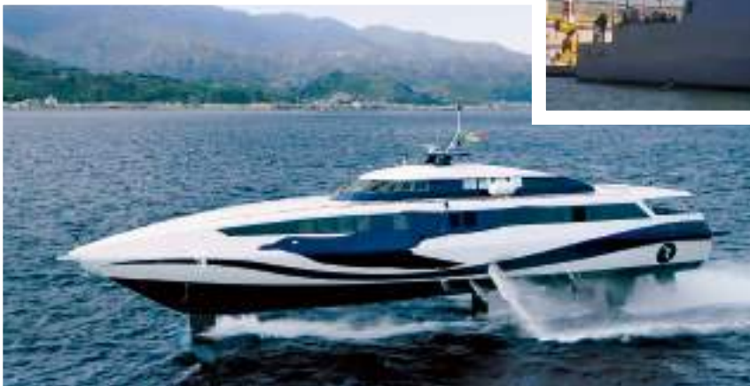
Fully Submerged Wings Hydrofoil: FSWH 37
