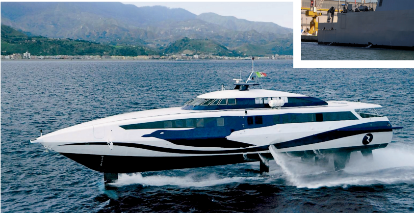
Fully Submerged Wings Hydrofoil: FSWH 37
